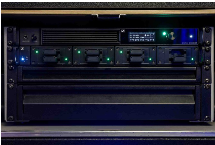
The Spectera Base Station, an L 6000 charging station and two drawers for the SEKs and accessories – the Spectera wideband system takes up hardly any space
